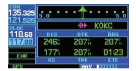
Turn the small **left** knob to select the desired kilohertz (kHz) value. For example, the '.80' portion of the frequency '117.80'.
