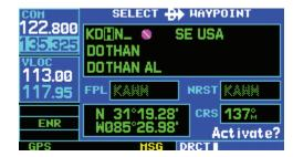
Press the ENT Key to confirm the selected waypoint, and press the ENT Key again to activate the direct-to function.
