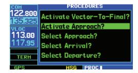
The 'Activate Vector-To-Final?' option allows the pilot to activate the final course segment of the approach. This option assumes the pilot will receive vectors to the FAF and provides guidance to intercept the final course, before reaching the FAF.
