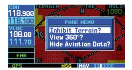
2) Press the **ENT** Key. The 'TER INHB' annunciation is displayed in the TERRAIN annunciator field when TERRAIN is inhibited.
