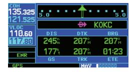
4) To activate the selected frequency, press the **COM Flip-flop** Key for COM frequencies, or the **VLOC Flip-flop** Key for VLOC frequencies.
