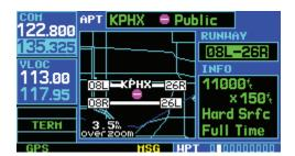
6) To view the other airport information pages, press the small **right** knob to remove the flashing cursor and turn the small **right** knob to select the desired page.
