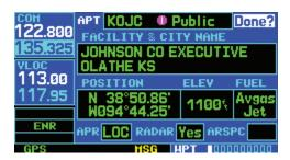
airport (including the airport runway and airport frequency pages), press the small **right** knob to remove the flashing cursor. Turn the small **right** knob to display the additional WPT pages. When finished, press the small **right** knob to return the flashing cursor to the screen.
