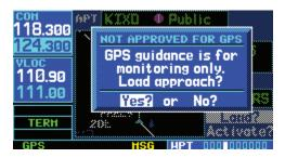
Not all approaches in the database are approved for GPS use. As the pilot selects an approach, a 'GPS' designation to the right of the procedure name indicates the procedure can be flown using the GPS receiver. Some procedures do not have this designation, meaning the GPS receiver may be used for supplemental navigation guidance only. ILS approaches, for example, must be flown by tuning the VLOC receiver to the proper frequency and coupling the VLOC receiver to the external CDI (or HSI).
