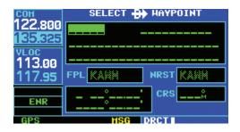
Use the small and large right knobs to enter the identifier of the desired destination waypoint.
