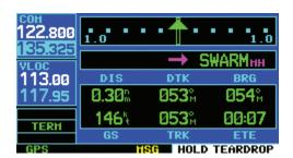
The GNS 430 provides course guidance only on the inbound side of the holding pattern. When leaving the holding pattern to re-fly the approach (or another approach) press the PROC Key to 'Select Approach?' or 'Activate Approach?' as previously described. (Or, use the Direct-to Key to select another destination.)
