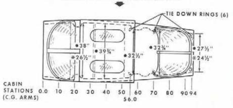
Figure 6-5. Internal Cabin Dimensions
