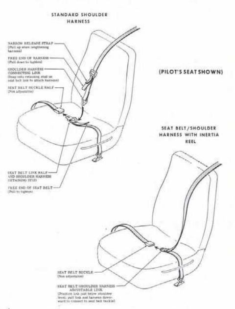
Figure 7-4. Seat Belts and Shoulder Harnesses
