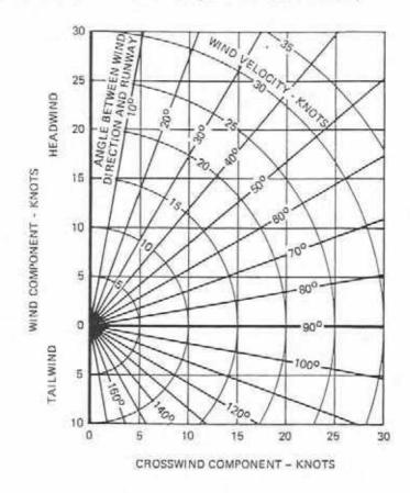
Figure 5-4. Wind Components
